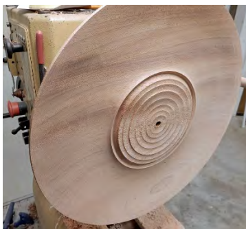
Photo 13 - Recess cut with parting tool at outer edge of depression
