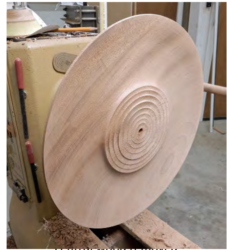
Central wood removed
