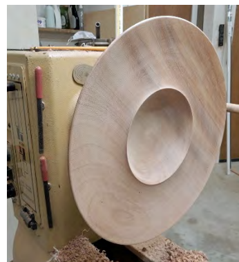
Photo 14 - Inner depression completed
