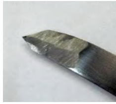
Photo 15a – Very thin parting tool made from a butter knife
