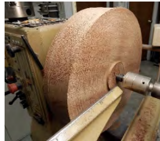
Photo 4 - 1/4 inch tenon cut
