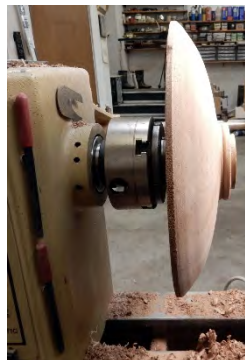
Photo 8 - profile of bowl bottom, base, and tenon
