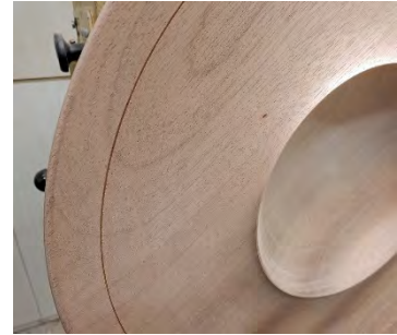
Photo 16 – Thin, shallow groove cut with butter knife parting tool
