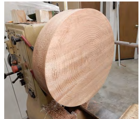
Photo 2 – Bowl blank mounted on a screw chuck and trued
