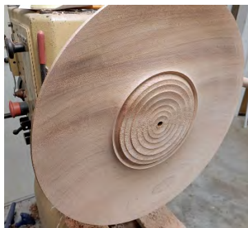
Photo 13 - Recess cut with parting tool at outer edge of depression
