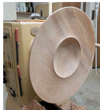
Photo 14 - Inner depression completed
