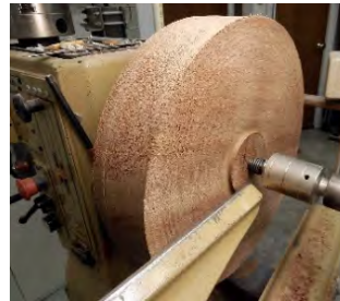
Photo 4 - 1/4 inch tenon cut
