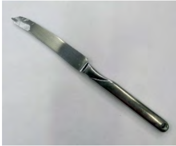
Photo 15a – Very thin parting tool made from a butter knife
