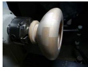
Finish-turn the outside and inside
