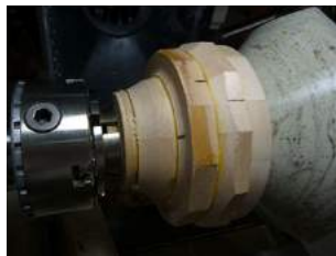
Glue all rings together concentrically
