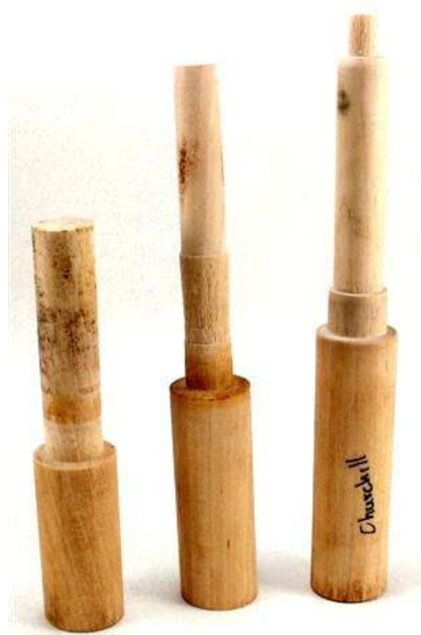
Wooden jamb chucks as explained above.
