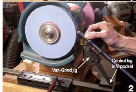
For best control of sharpening, hold the Vari-Grind in your hand. Avoid attempting to control by gripping the tool handle.
