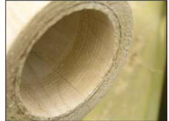
Sand the edge that the liner's lip is going to cover and get everything to fit correctly. The liner should fit snugly, but still allow you to pull it out. Turn the remainder of the blank down to size. The inside doesn't have to be perfectly smooth. The liner will hide any roughness left from the hollowing process.
