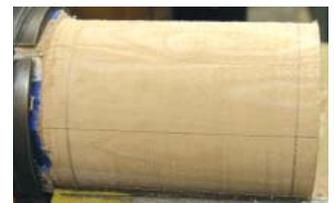
With the block squared up, mount in either a chuck or a faceplate. This project is an end grain mounted turning, so screws won't have as great a holding strength as they would in cross grain. It is also important to use all the available holes in the faceplate and screws with sufficient length.
