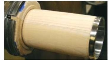
If any hollowing was done where the mug was parted off, slide the liner onto a jam chuck or use your chuck jaws, spread out from inside the mug's opening, to hold the blank in place to clean up the inner diameter of the bottom. Bring the tailstock up in support for using a scraper or gouge to lightly clean up the plug edge. Fit the plug and glue into place. Once dry, re-chuck as above and turn any excess off the bottom using light cuts.
